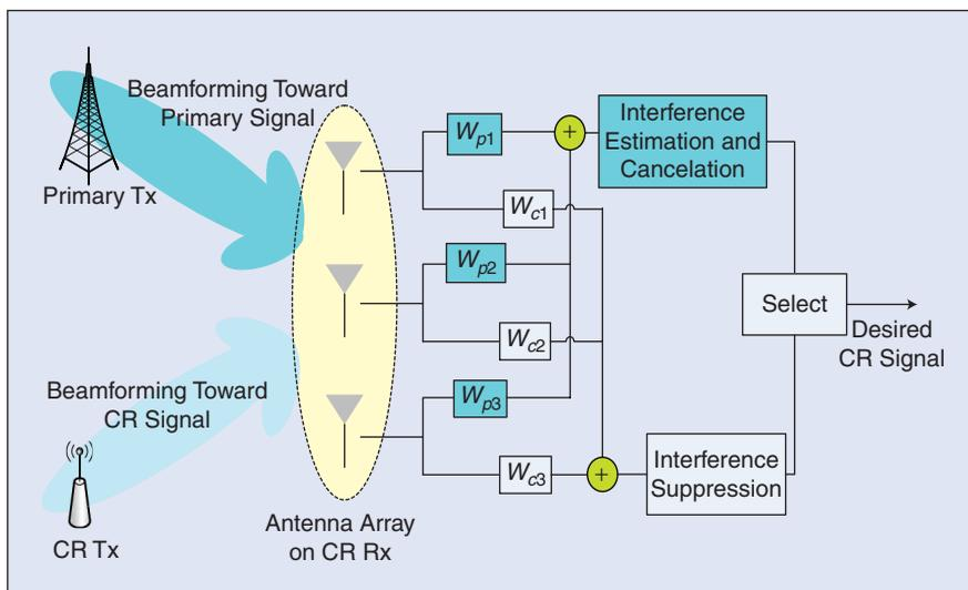
**FIGURE 5** A hybrid IC technique combining beamforming and interference cancellation/suppression.
