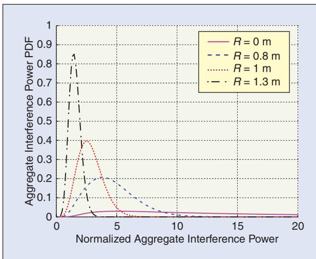
**FIGURE 2** PDFs of the aggregate interference power (normalized to the transmit power of the interferers) with different values of the exclusion region radius  $R$  (CR transmitter density  $\lambda = 1$ ).
