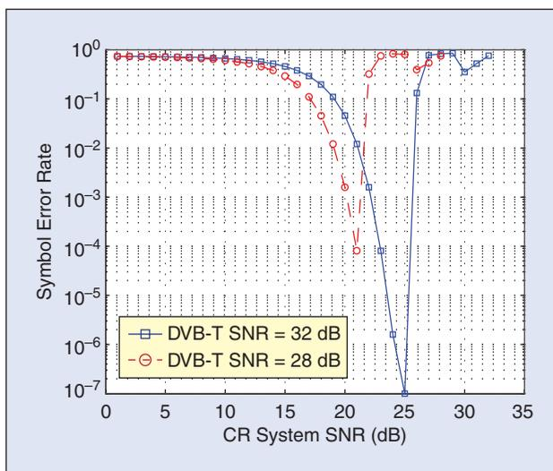
FIGURE 4 Symbol error rate performance of a CR communication link in the presence of high-power interfering DVB-T signals.
