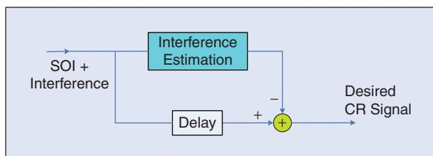
FIGURE 3 Block diagram of a CR receiver using interference estimation and cancellation.
